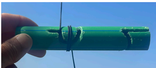
5. Wrap the line two rounds over the "tongue".
