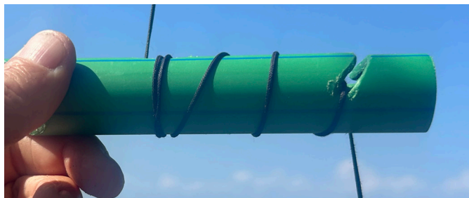
7. Slip the line into the second cut-out slot and wrap the line one and a half round inside the second cut out sling.
