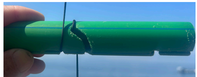
4. After the "tongue" has caught the kite line, the line exits the cut-out in the opposite direction.
