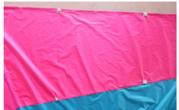
Batten pockets (blue) and spine sleeves (red).
