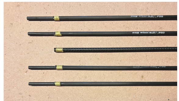
Skyshark tubes with long internal ferrule and end reinforcement.
