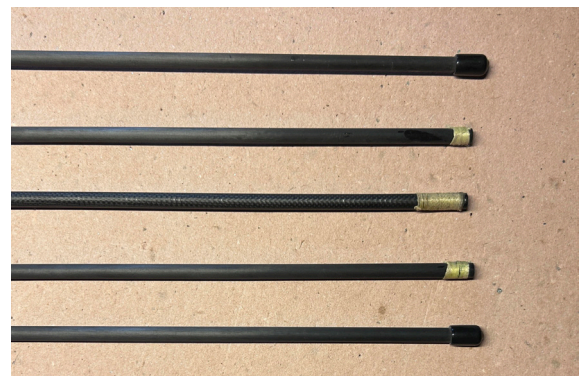
Skyshark tubes with long internal ferrule and end reinforcement.
