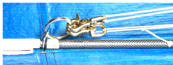
String tension anchor system in the middle of the halved middle tube.
