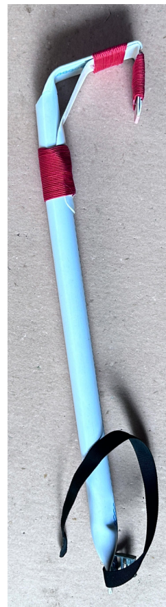
Collapsable fishing rod with T connector in top. There are removable carbon tubes inserted in the top T connector to prevent kites accidentally blowing off the rod prematurely.
