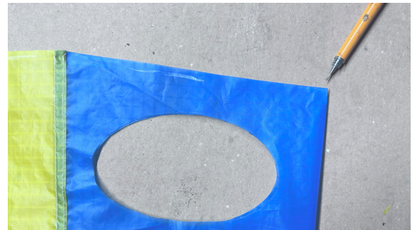
Roof part folded over wall part for second seam and corner trimmed.
