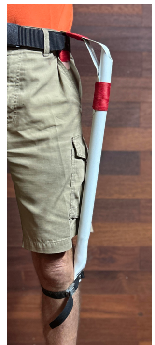
Since PVC material is rather flexible, the hook has been reinforced with the flattened 'half pipe' sawed off in step b.
