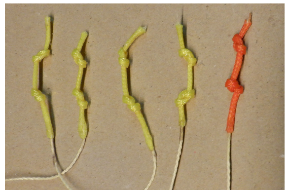
The five pieces of sleeve with two figure-of-eight knots acting as stoppers.
