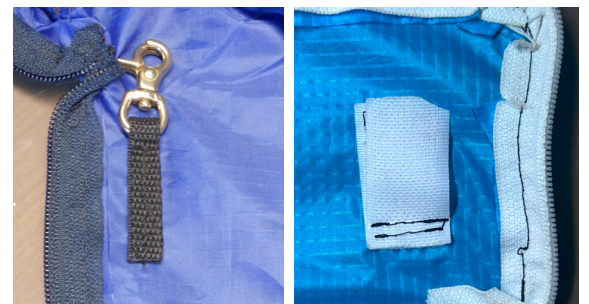
A lobster hook or a piece of velcro for the start of the train line (from the bottom element in the train), easy to open with one hand, and located out of the way in a corner of the top lid.
