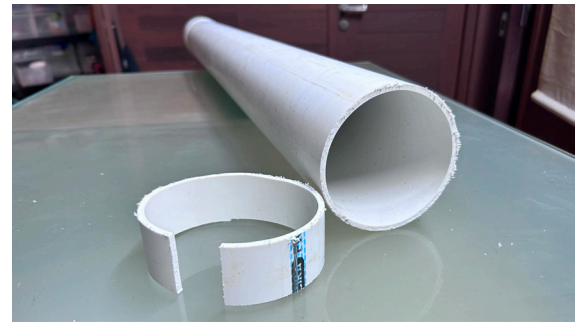
PVC tube, 4" (11.4 cm) Ø, with a 4 cm cut off piece to make a spool holder.
