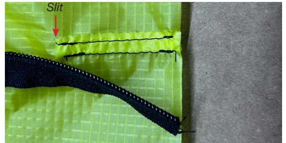
1 cm slit with fold over seam.
