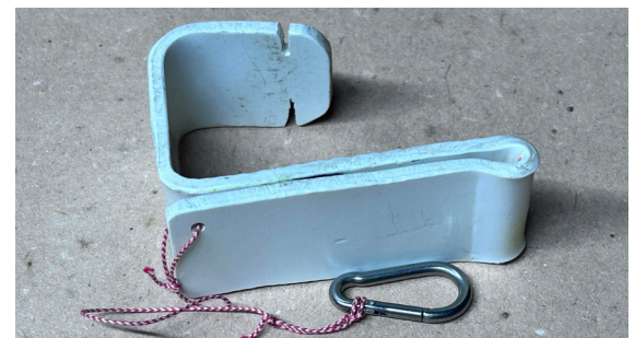
To avoid that the spool holder slips off the belt and gets lost, a lanyard with a carabiner can be added to the spool holder.
