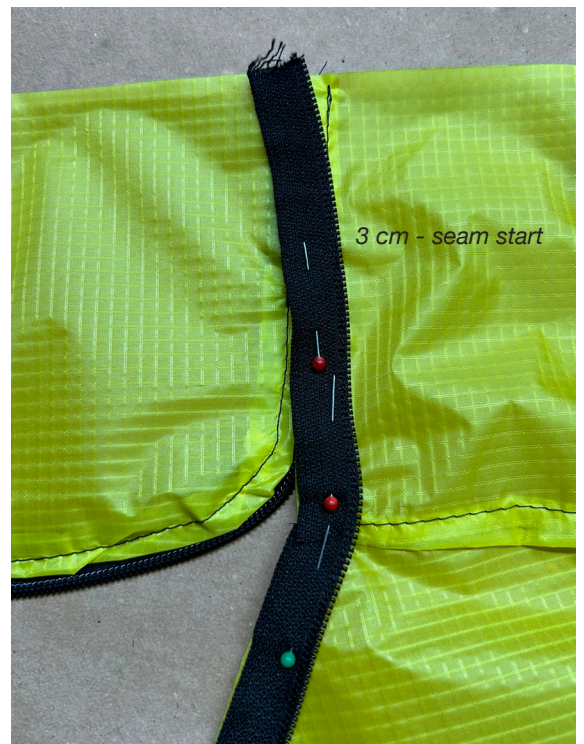
1 cm slit with fold over seam.
