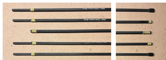
The inwards ends of the cross bow P90 tubes with the stiffer P2X in the middle (without internal ferrule).
