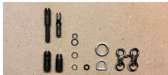
Alternative details for the tensioning anchor system. From left: split endnock (1), small split ring or small solid ring or small 8 ring (1), small rubber ring (1), O-ring or D-ring (1), lobster claw hooks (2).
