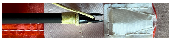
Tubes joined with an 8 ring around the internal ferrule and an O ring tied to the 8 ring. The bent part of the 8 ring facing the spilt end nock.
