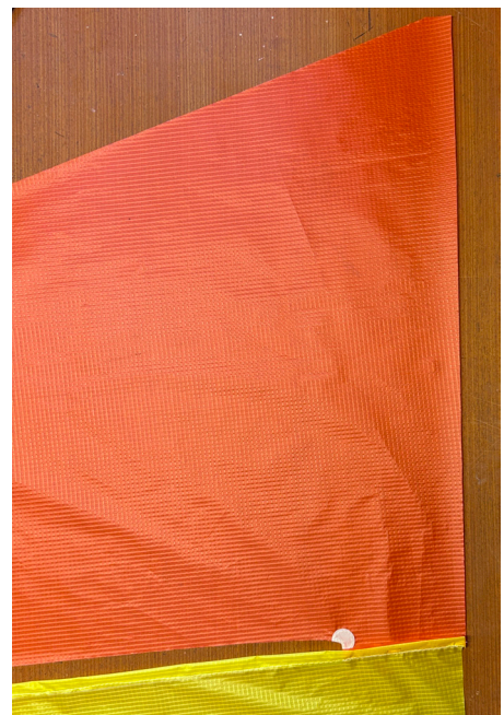
First seam along the edge of the sleeve (below the sleeve seam).
