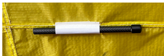
The sleeves must be tight in order to keep the spine tube firmly in the correct position sideways, but still wide enough to let the tube with end cap go through.
