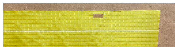
4b. Exit hole for 3 mm tube/rod 6 cm from the spine edge.
