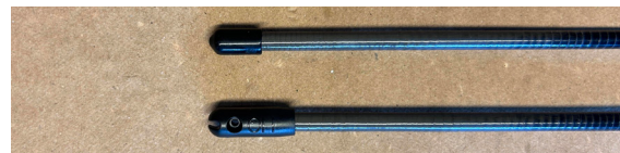
Tube for the spine: one with internal ferrule and both with reinforced ends.
