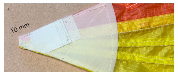
Alternative pockets for cross spar on wing tip. The lower corner of the pocket has been trimmed with the sail wing tip edges.
