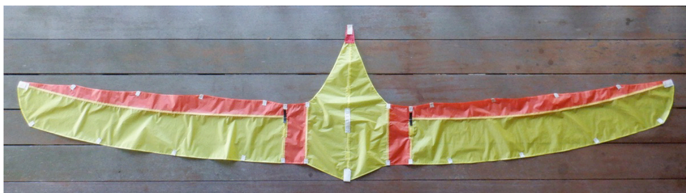
Entire wing sail complete with pockets and reinforcements.
