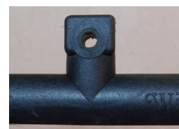
The spine hole/stand-off rod hole stepped down from 6 mm to 4 mm.
