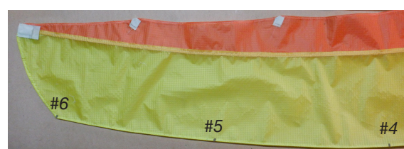
Position marks for rear pockets for battens #6, #5 and #4. (#3 not shown in picture.)
