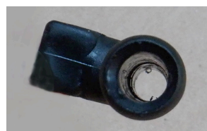
Spreader separator of cross connector A drilled through with diameter for centre Skyshark tube.
