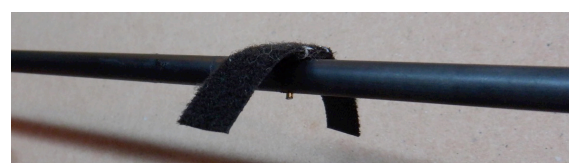
Nail protruding 1 mm.
