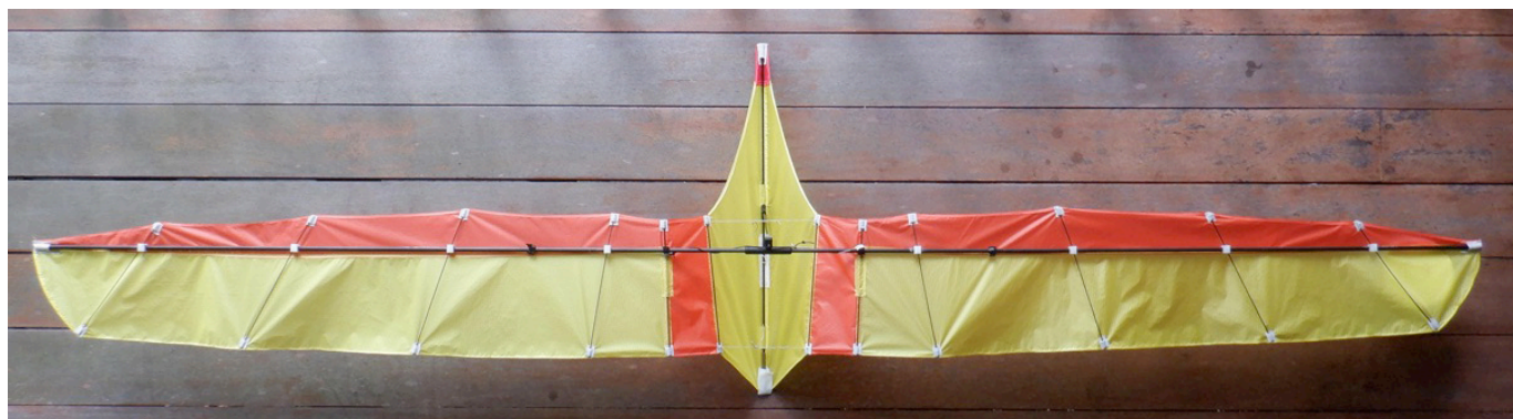
The completed kite with tensioned leading edge and bulging trailing edge.
