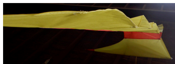
Side view: The trailing edge is bulging upwards in the air and create dihedrals around every batten.
