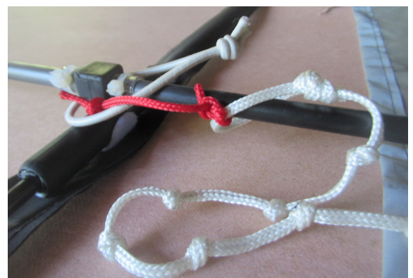
5 cm securing string (red) hold knotted string and bungee in place. Bungee released for clarity reasons.
