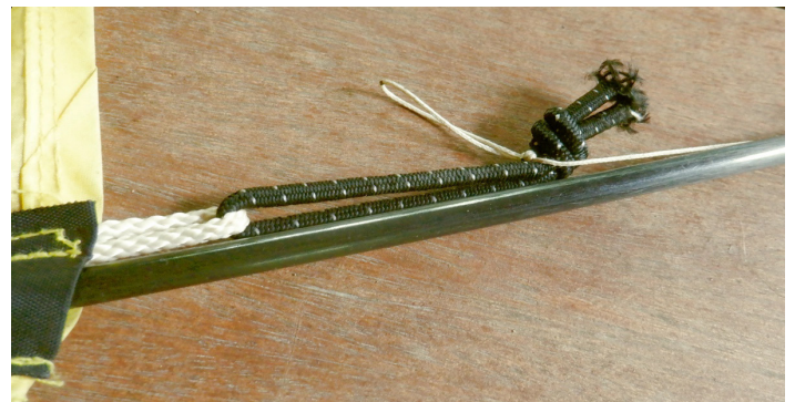
Complete wing tip with tension strings wrapped around the spars
