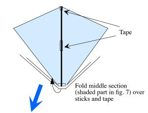
**9.** Make four sticks that have the same length as the <u>width</u> of the kite. Take two at a time and make up into two bundles. Use adhesive tape at the end of the bundles and at three places with equal distance in between along the bundles. Fix the bundles across the kites with adhesive tape. At the short end let the tape go over the edge to the other side of the sheet. Don't tape in the middle!
